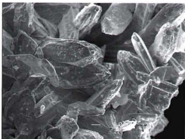
Figure 8. Flattened pointed scotlandite crystals up to 0.05 mm long from Lady Anne Hopetoun Shaft. Tim Neall collection.
