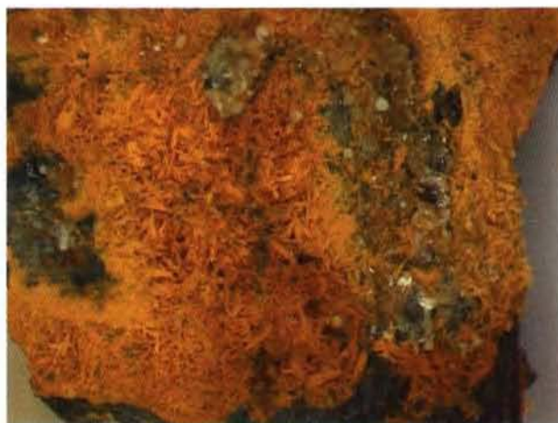
Figure 3. Hydronium jarosite pseudomorphs after prismatic gypsum crystals with colourless gypsum overgrowth. National Museum Wales specimen no. NMW 2006.11G.M.6. Field of view 9 mm across.
