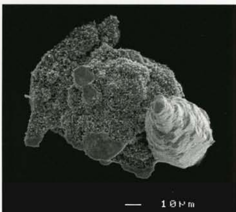
Figure 5. A spindle shaped arsenatian vanadinite crystal on platy phosphatian mimetite, which is covered in minute sharp plumbogummite crystals.
