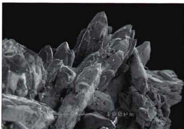
Figure 12. Blocky pointed Type 1 scotlandite crystals up to 0.1 mm long from Whitwell quarry. Peter Briscoe specimen.
