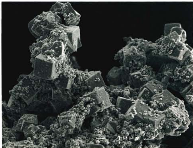
Figure 15. Blocky pseudo-cubic beudantite crystals up to about 20 \mu\text{m} across from the Howthwaite trial.
