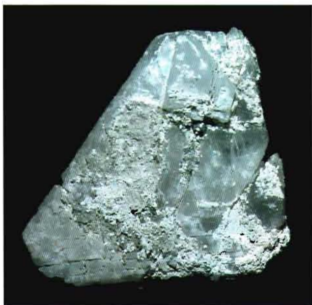
Figure 3. Baryte crystal, fractured and re-cemented with alstonite and witherite. Admiralty Concession Flat, 2nd Sun Vein, Nentsberry Hags Mine, Nenthead, Cumbria. Specimen width 15 cm.
